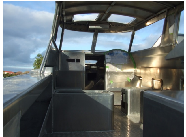
The Kiribati Islands safety boat ready for painting
